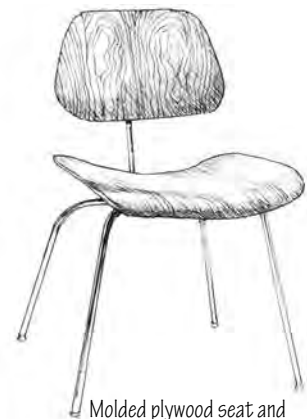
Molded plywood seat and back with a steel frame— Charles Eames
